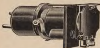
FIG. 133.—Sterling Line Drop, showing the centrally swung armature and the restoring slide in front.
